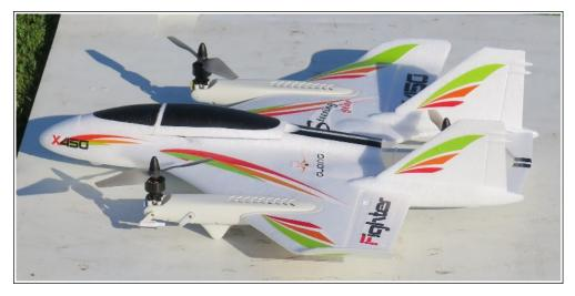
It has three basic modes, hover like a drone, vertical attitude (pointing straight up!), and fly like a plane. In the
